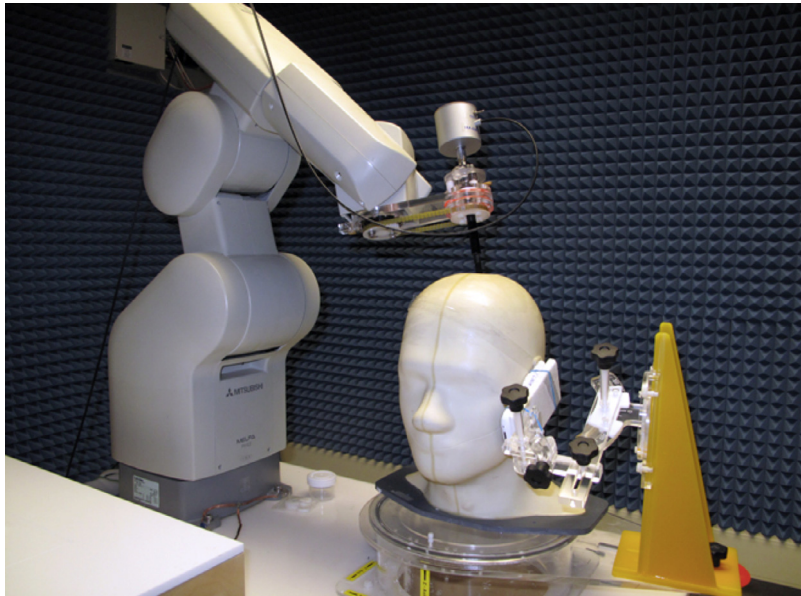
Fig. 6. Cell phone SAR RF test system using Specific Anthropomorphic Mannequin Model.
